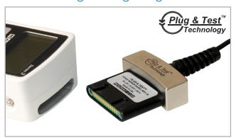
^ Unique Plug & Test™ technology allows for interchangeable sensors to be used with a Mark-10 model 7i, 5i, or 3i indicator. All calibration and configuration data is saved in the smart connector.
