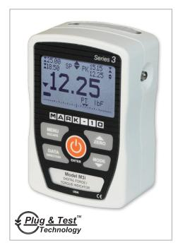
The 3i digital force / torque indicator is designed to work with a wide range of Mark-10 remote force and torque sensors (see page 3). With exclusive Plug & Test™ technology, all calibration and configuration data is saved within the sensor's smart connector, not the indicator, allowing for true interchangeability. In addition, all sensors are fully compatible with other Mark-10 indicators.
